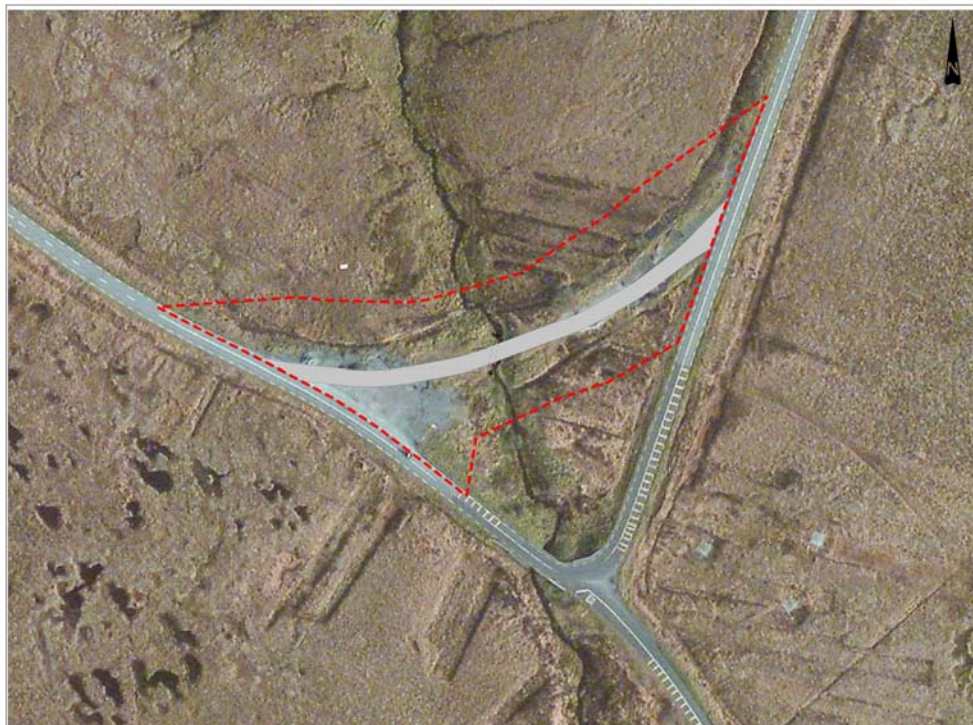
Figure 4 Image showing proposed crossing location – note disturbed state of the bog at bridge location as a result of previous ground works and previous cutting.
